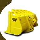
Built to withstand harsh environments and severe service, Heavy Duty Rock Buckets are reinforced with extra thick plate and AR 400 wear protection on all wear surfaces. Straight, semi-spade and full spade edges available with your choice of teeth and segments. Features a plate style spill guard.
