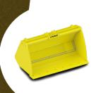
The Craig Ejector Bucket is designed to allow for easy loading and unloading of materials where dump height clearances are a challenge. The back of the bucket is hydraulically activated and swings forward ejecting the material outwards. Allowing for controlled dumping scenarios along with reducing the need to raise the bucket up and emptying using the loaders dump/tilt cylinder function.
