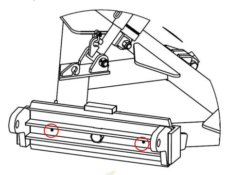
If a trip edge is installed, the complete trip spring assembly should be greased daily, especially the shaft that is inside the spring.
