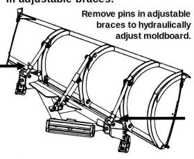
Replace pins in adjustable braces before using plow
