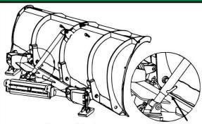
Use adjustable brace or cylinder to adjust cutting edge angle. RECOMMENDED ANGLES:
