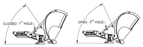
When in heavy snow conditions or when peeling hardpack, opening the moldboard to the 63° position is recommended. This position will make the plow scrape better, but consequently will make the moldboard jump or trip easier when hitting obstructions and the moldboard may chatter.
