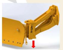
When plowing snow with the Craig 300 series wing, the front post should be fully lowered. This will allow the wing to float approximately 5" down and 7" up. The rear lift (connected to a valve section equipped with float capability) must be operated in the float position. Doing this will allow the Craig wing to follow any imperfections in the road surface. Also, if an object is struck while plowing, the wing will float over the obstacle to avoid damaging any
