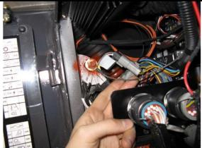
Locate a suitable ground connection to ground the control box.
