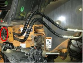
3. If there are hoses for AWD running along the right-hand side of the cab, they will need to be rolled up to make room for the front lift assembly.
