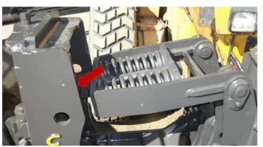
In order to adjust the spring tension, the pin must be removed connecting the brace to the rear of the slide assembly (indicated by RED arrow above).
