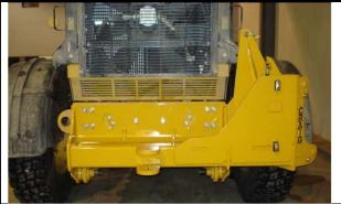
12. Mount the rear post bracket (RPB) to the rear bumper using provided bolts and washers. DO NOT damage hydraulic adapters.
