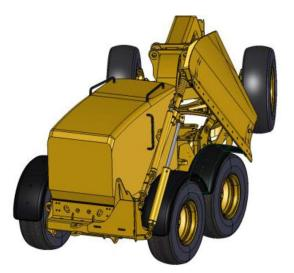
In order to articulate the grader and know that there will be no unwanted contact with the grader the wing needs to be either fully raised (front and back) or on the ground plowing snow. The design of the 300 series, in one of these two (2) positions, will allow the grader to have the full range of motion whether the machine is articulated (left or right) or is being articulated... See below for important notes.
