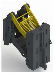
Adjusting the tension should only be completed in a controlled environment, and only if it is absolutely necessary. The trip springs are pre-tensioned to approximately 2500 lbs when they leave the factory.
