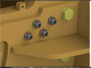
14. Install bulkhead adapters for the rear lift hoses in the RPB.
