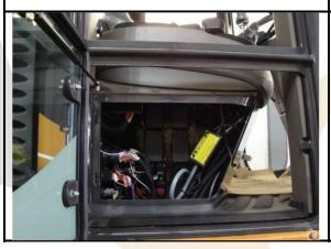
Replace the cover on the control box and install the supplied decal on top of the box. The joystick installation is complete. If you encounter any problems or have a suggestion about something that may not have been clear in this manual please feel free to call us toll free at 1-800-565-5007, or send us an e-mail at
