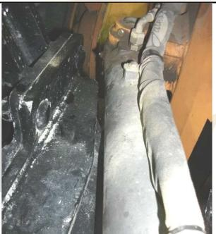
7. Ensure that the machine can be fully articulated to the left and that there is clearance between the bracket and articulation cylinder.
