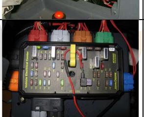
Locate an existing fuse (keyed power) less than 10A. Install the "Add a Circuit" according to the instructions printed on the package and both the existing and the new fuse will work independently.
