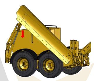
When lowering the wing to start plowing, the front post will lower much faster than the rear of the wing. A good practice to get into is to lower the rear of the wing prior to lowering the front.
