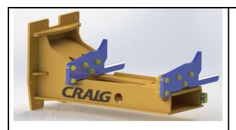
5. If the FPB cannot be bolted directly to the grader it will have weld on pieces such as shown in blue in the picture to the left. They weld to the bottom of the grader near the articulation point. Ensure that the mounting plates are bolted securely to the FPB, so they won't move while tacking in place under the machine.
