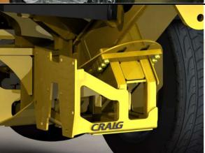
4. If the front post bracket bolts directly to the belly pan of the grader, visually check the holes to ensure they can freely accept the bolts. Mount the front post bracket using supplied bolts and washers. NOTE: It will be easier to handle and mount the front post bracket (FPB) with the lift group disconnected.
