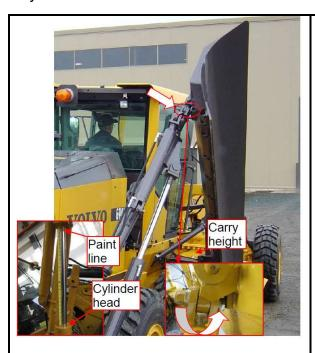
Following this procedure is the responsibility of the installer and will ensure that when the wing is being transported in the carry position there is no excessive "slap" or movement in the wing, which may cause premature damage to the equipment. This procedure should be repeated periodically or as required.
