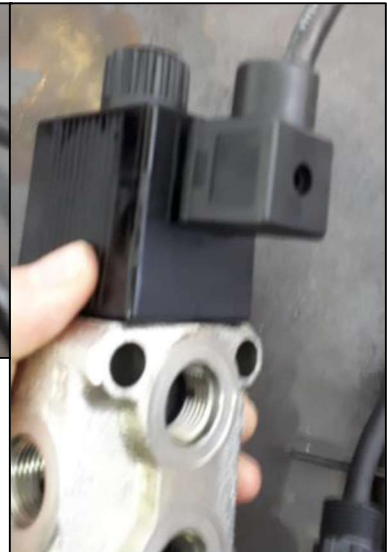
Figure 4: DIN Connector Attached to Diverter Valve
