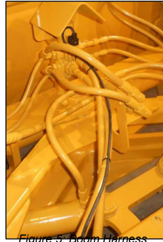
Figure 5: Boom Harness Routed on Hoses
